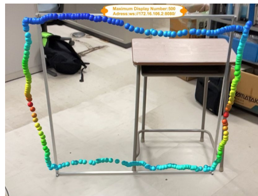
Figure 6. Accuracy evaluation for freehand tracing on a square area. The length of a side is 900 mm.
